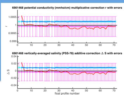
Figure 4: Correction proposed by the OW method for Deep-Arvor floats 6901468 (identified by blue stars on Figure 1). (Upper panel) The red (blue) curve represents the conductivity correction term for each profile while the magenta (cyan) line is the final correction term with one standard error when considering layers shallower than 2000 dbar (layer deeper than 3000 dbar). (Lower panel) Same as upper panel but for the vertically averaged salinity correction.
