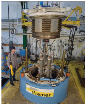
Figure 1 : Qualification en pression des tubes (composites) Deep-Arvor.
